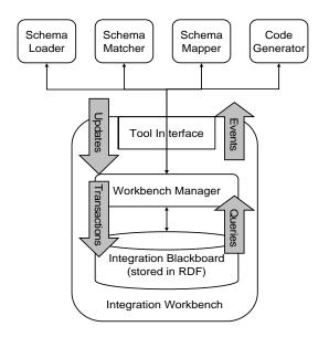
Figure 8: Integration workbench architecture.
