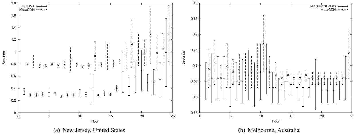
Figure 8. Direct replica access versus MetaCDN Load Redirection
